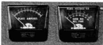
Continuous monitoring of Ip plus switch selected monitoring of Rel Pwr., Ep & Ig.
